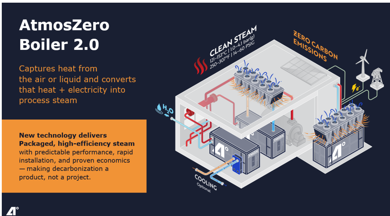
Diagram 1 – AtmosZero Steam Heat Pump in Various Heat Source Configurations
